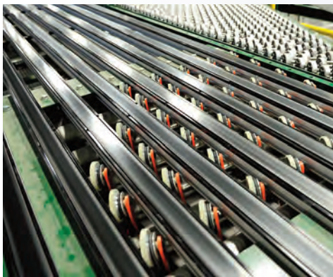
A Narrow Belt Sorter with 30 degree diverts that pop up in a wave fashion.
