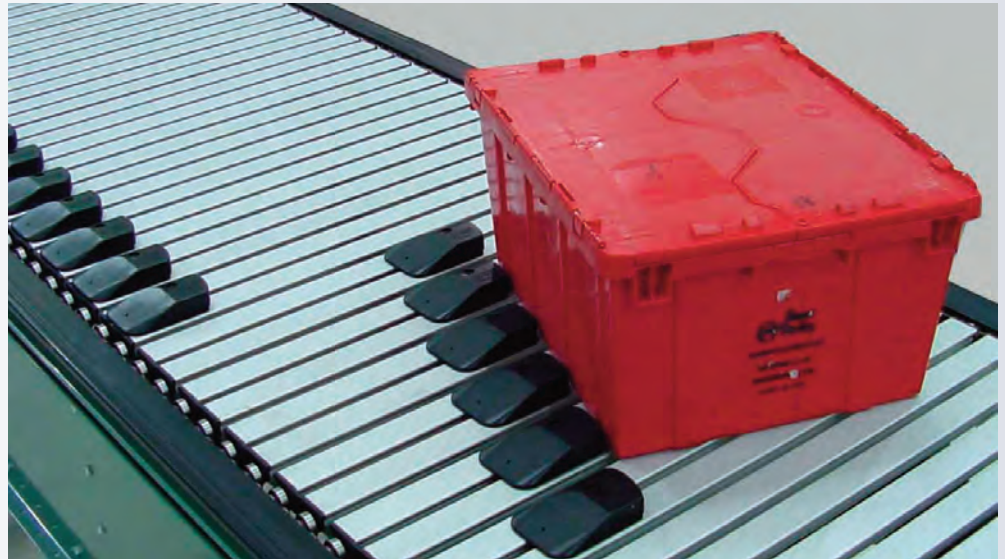
A tote being diverted on a sliding shoe sorter.
