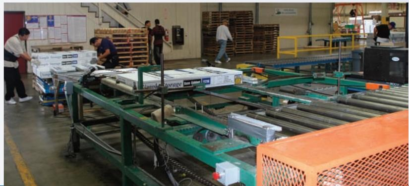
A gravity conveyor routes cartons to an adjustable height lift table so workers can utilize manual palletizing methods.
