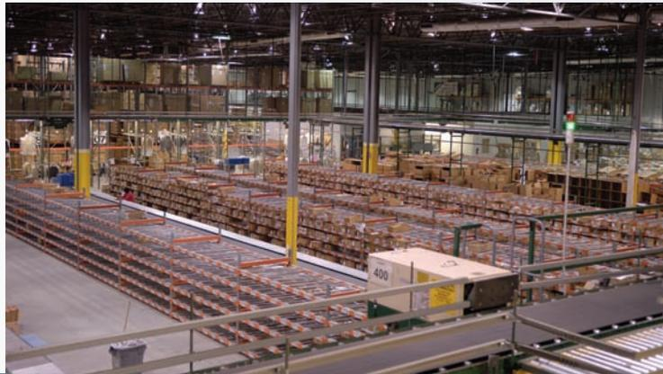
An overview of a well-planned distribution center, showing an overhead conveyor with an integral “pusher” sortation device and shelving setup for an “each” or split-case picking operation. In the far background is double-deep pallet rack storage lift table so workers can utilize manual palletizing methods.
