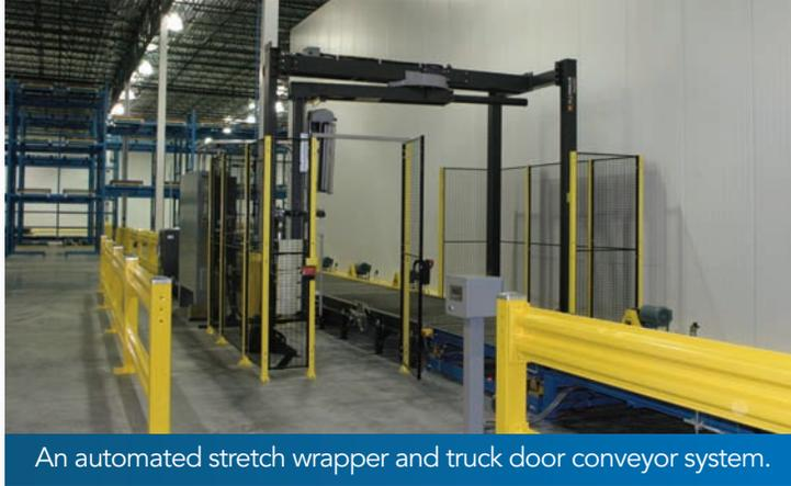
An automated stretch wrapper and truck door conveyor system.
