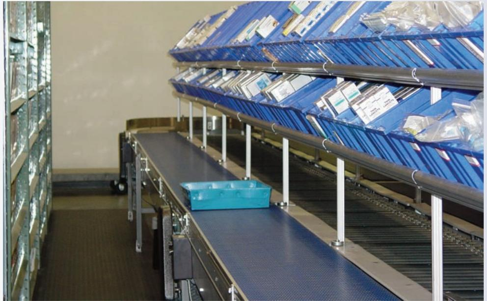
A tote enters a pick zone via a blue table-top plastic chain conveyor. Once the tote is picked, the picker slides it onto the 24V MDR takeaway conveyor en route to pack-out and shipping.
