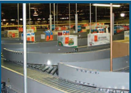
*Multiple lines from different picking areas are merged in stop/route order prior to induction to the shoe sorter.*
