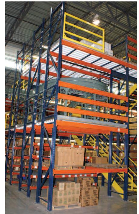
*The north end of Mecalux 3-level pick module. The 1st level is used for picking from carton flow rack, 2nd & 3rd levels are used for picking from pallets.*
