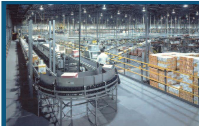
Cases are scanned prior to 180-degree curve and then are tracked until they reach sort destination and are diverted down to dock doors.
