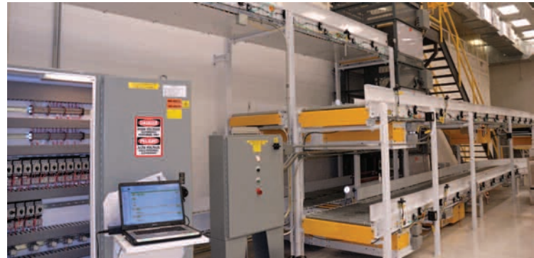
Vertical lift conveyor delivering ingredient totes to three levels of zero pressure accumulation conveyor and to each respective mixer while conserving essential floor space.
