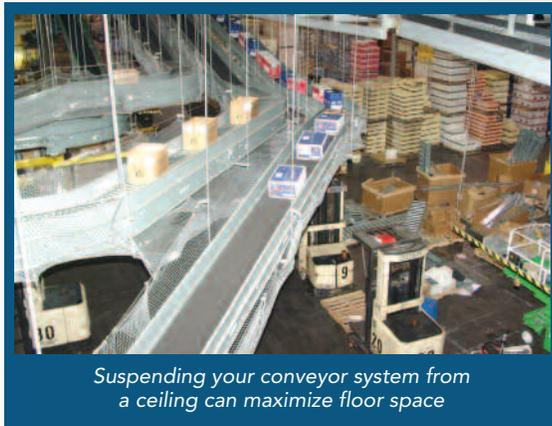
*Suspending your conveyor system from a ceiling can maximize floor space*
